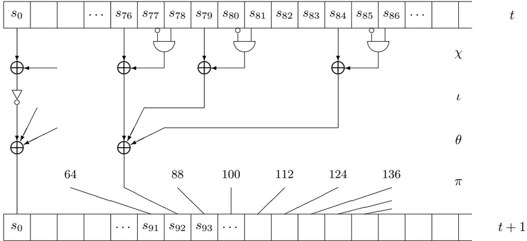
Figure 1: Subterranean round function, illustrated for bit  $s_{92}$
