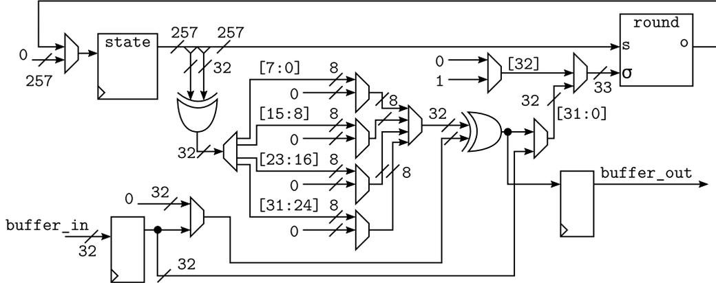
Figure 4: Subterranean round with registers and duplex logic.
