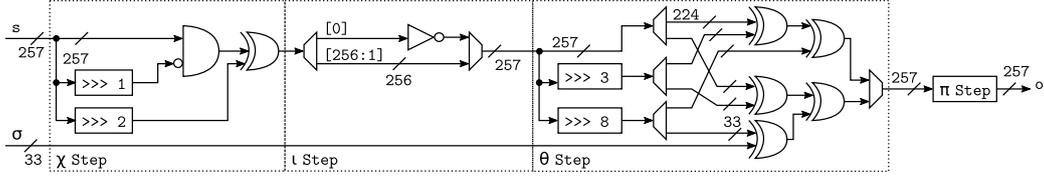
Figure 3: Subterranean round hardware architecture.
