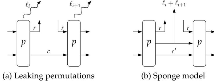
Figure 4.1.: Leakage of information in sponge-based constructions.
