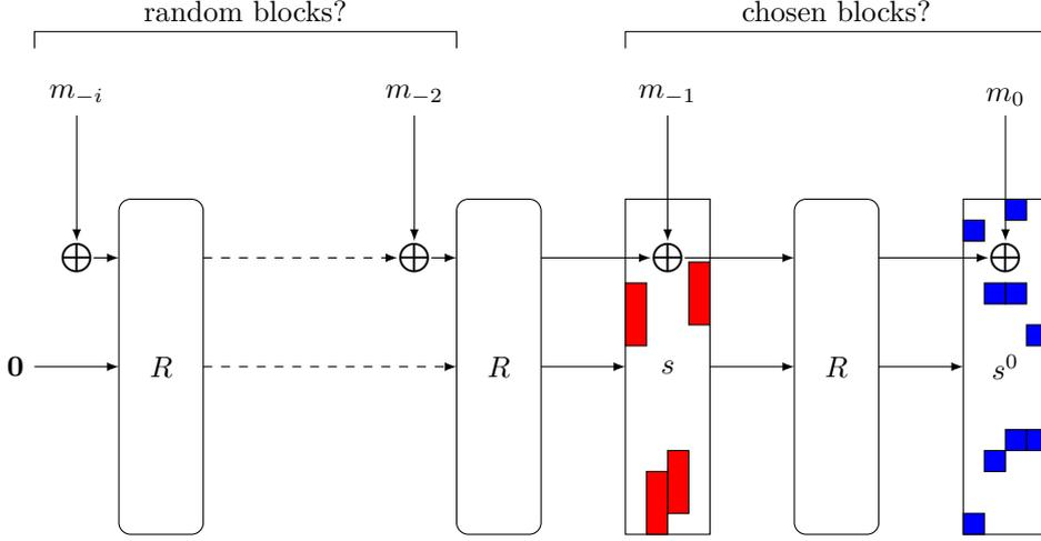
Figure 2: Finding state collisions in unkeyed absorbing. We want a collision on  $s^0$ , bits in blue are *input block bits*, only their difference matters. Bits in red represent conditions that can be satisfied by choosing the value of  $m_{-1}$ , where  $m_i$ 's are message blocks concatenated with the padding bit.
