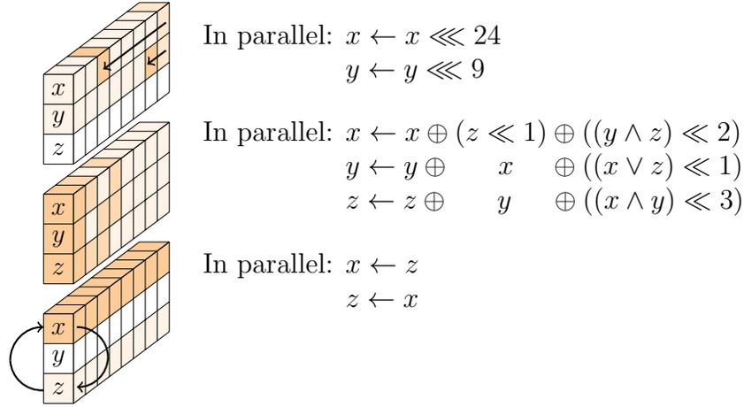
Figure 2: The SP-box applied to a column
