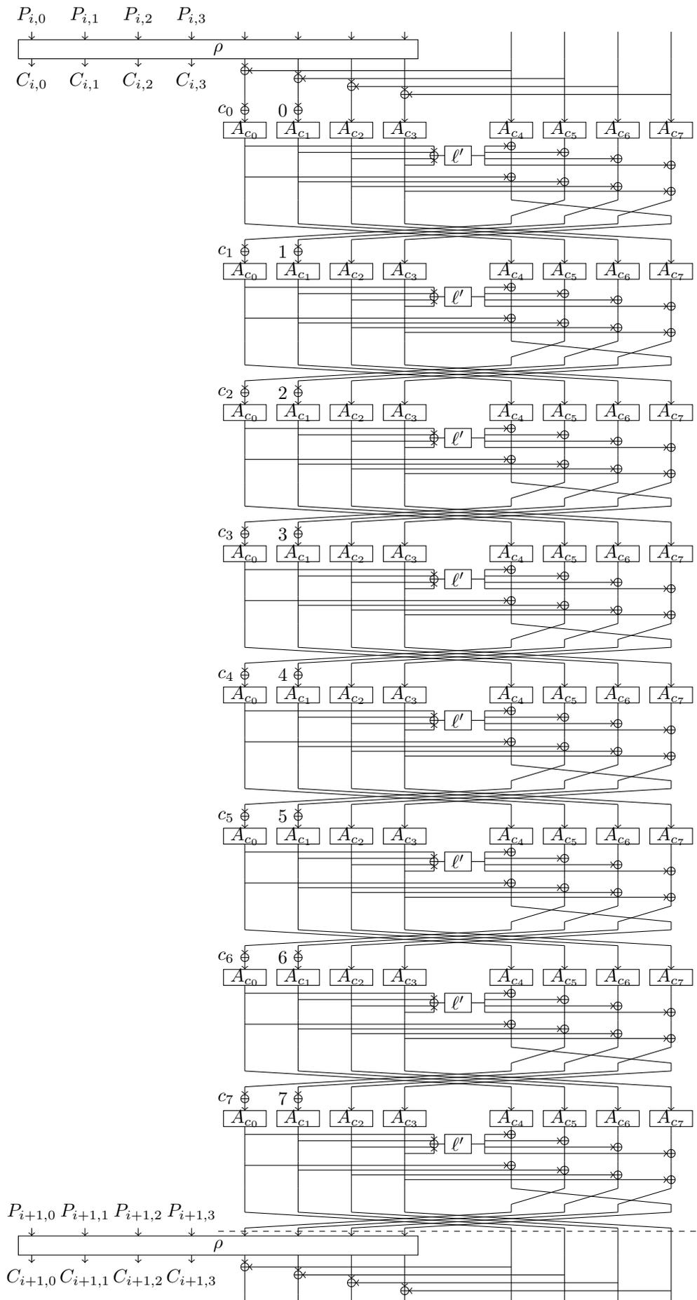
Figure C.7: High-level structure of SPARKLE with 8 steps.
