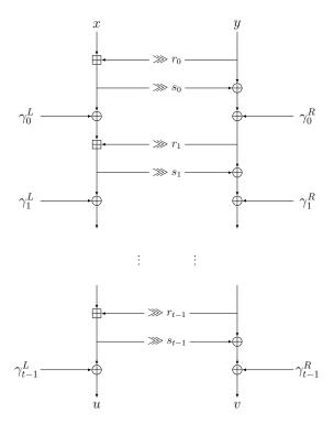
Figure 3.3: The general structure of Alzette.
