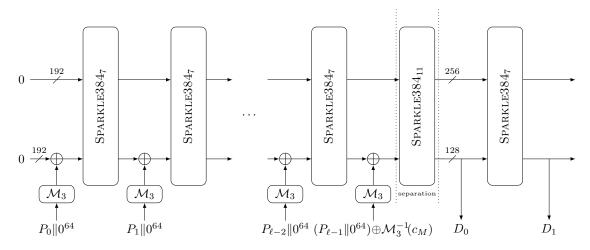
Figure 2.3: The Hash Function ESCH256 with rate r=128 and capacity c=256. The constant  $c_M$  is equal to  $(0,0,\ldots,0,1)\in\mathbb{F}_2^{192}$  if the last block was padded and equal to  $(0,0,\ldots,0,1,0)\in\mathbb{F}_2^{192}$  otherwise.
