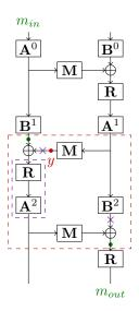
**Precomputation/Data Trade-off Attack.** Note that the left part of Equation 4.3 is independent of  $m'_{in}, m'_{out}$ . Moreover, the right part consists of independent ARX-boxes. Therefore, guessing one 64-bit branch of y leads to knowledge of an input and an output 64-bit branches of the function from the left-hand side. A data trade-off attack follows. The trade-off parameterized by an integer  $r, 0 < r \le 64$ .
