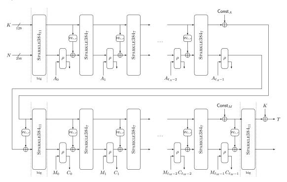
Figure 2.5: The Authenticated Encryption Algorithm Schwaemm256-128 with rate r=256 and capacity c=128.
