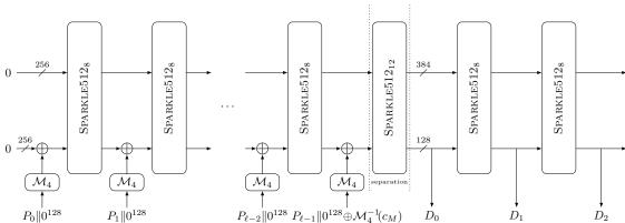
Figure 2.4: The Hash Function ESCH384 with rate r=128 and capacity c=384. The constant  $c_M$  is equal to  $(0,0,\ldots,0,1) \in \mathbb{F}_2^{256}$  if the last block was padded and equal to  $(0,0,\ldots,0,1,0) \in \mathbb{F}_2^{256}$  otherwise.
