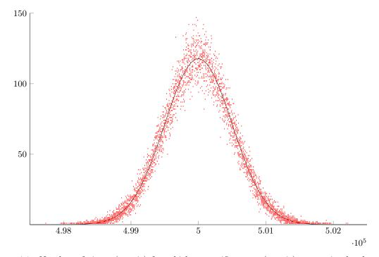
Figure 4.1: Number of times (y axis) for which a specific entry (x axis) occurs in the dependency matrix after three steps of Sparkle384 for  $10^6$  samples (red) and the theoretical number of occurrences corresponding to a  $B(10^6, \frac{1}{2})$  distribution (black).
